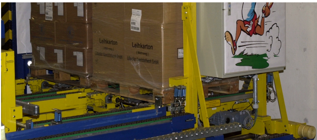
Displacing Device with double mounting pallets for automaticly stocking out incl. mounting. 110 pallets/hour; weight 1200kg; route 46m
