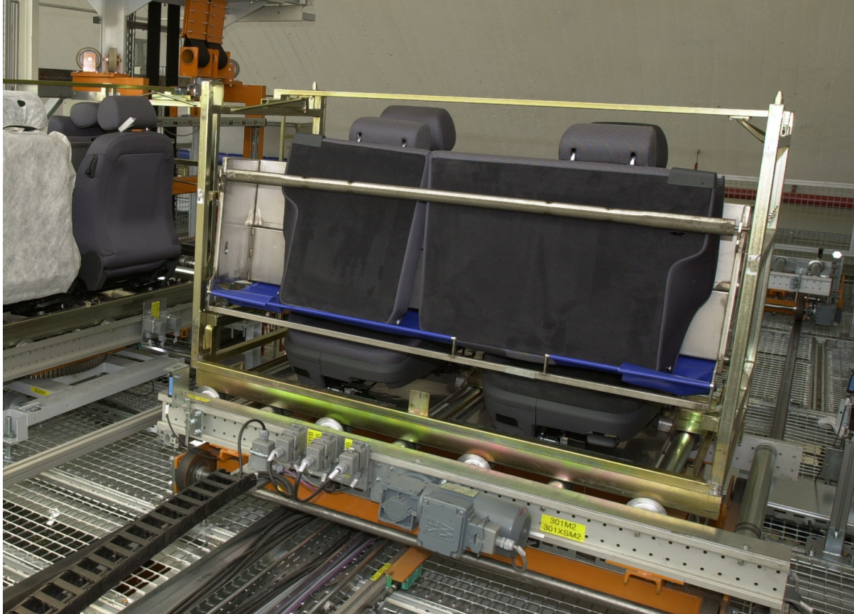
Displacing Device for complement Conveying tracks at the assembly line in the Automobil Industry
